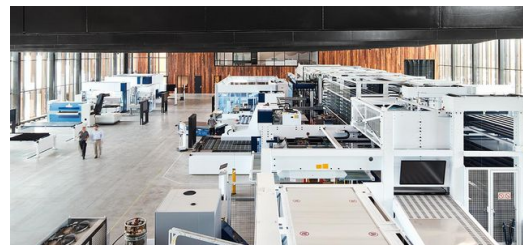
In a production hall measuring 55 meters in length, there is a connected sheet metal production with a central storage system as the centerpiece, which supplies the machine tools with material. (Foto: Steve Hall © Hall+Merrick)
