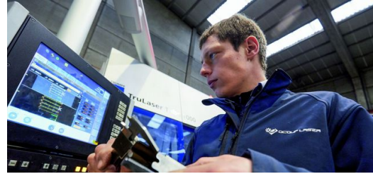
The simple operating concept behind the TruTops Tube software makes possible exact calculation of cutting geometries. Even complex calculations at the corners of rectangular profiles are automatically handled by this program. (Picture: Claus Langer)
