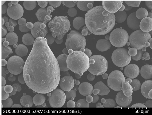
Figure 7: INNOFLEXX S900 powder by thyssenkrupp Schulte. PSD: 18-58 μm. SEM magnification: 600x.
