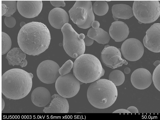
Figure 1: In625 powder by Oerlikon Metco. PSD: 15-45 μm. SEM magnification: 600x.
