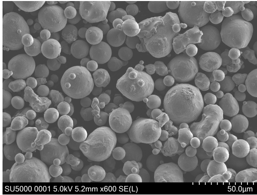
Figure 1: CoCrMo powder by Argen. PSD: 15-45 μm. SEM magnification: 600x.
