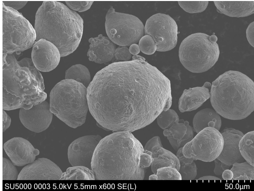
Figure 23: CP1 powder by Constellium. PSD: 20–63 μm. SEM magnification: 600x.
