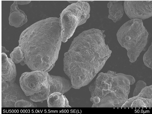
Figure 28: Custalloy powder by ECKA. PSD: 20-63 μm. SEM magnification: 600x.
