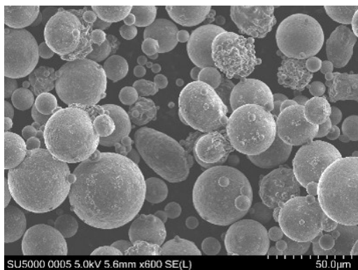
Figure 8: A20x powder by ECKART. PSD: 20-80 µm. SEM magnification: 600x.
