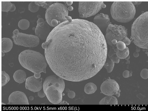
Figure 4: 6061-RAM2 powder by Elementum3D. PSD: 20-83 μm. SEM magnification: 600x.
