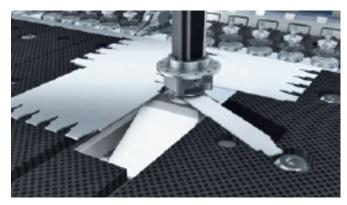
Clamping and rotating parts
