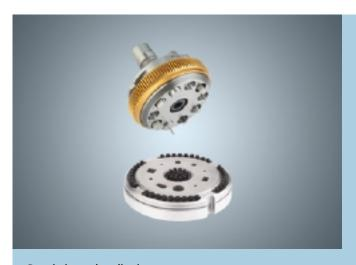
**Description and application**The original MultiTool from TRUMPF for optimal surface quality on the upper and underside of the sheet
