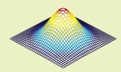
In the far field, the intensity distribution of the single-mode VCSEL is perfectly Gaussian shaped. The absolutely symmetrical and Gaussian-shaped beam profile makes the optical design of applications significantly easier.
