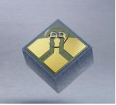
Chip die – two 850 nm VCSELs with single integrated photodiode (ViP) for high-volume self-mixing interferometry sensing applications and integrated speed sensors
