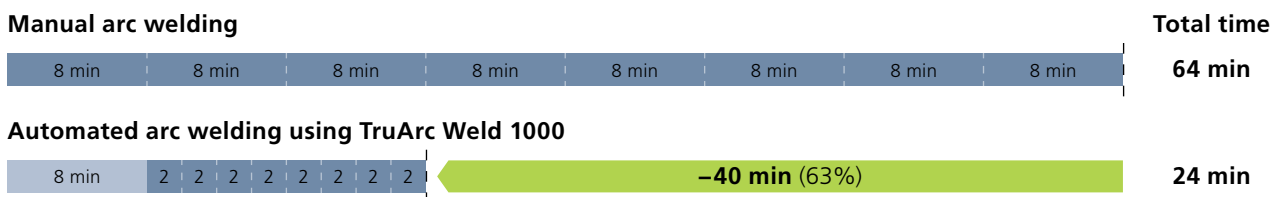
Shipping brace, 8 items with 10 weld seams.
