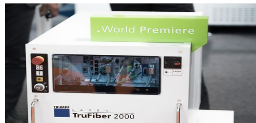
The fiber-based solid-state laser TruFiber 2000 celebrated its world premiere at the LASYS 2018. Because this laser has a compact laser design, flexible interfaces to all common fieldbus systems, and the maximum laser safety rating with Performance Level 'e', it also contributes to easy integration.
