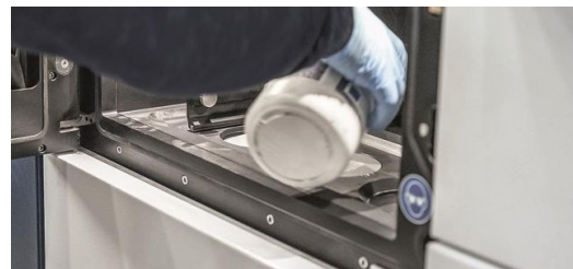
A healthy dose of powder: CONMET taps into the potential of 3D printing in two different ways. Firstly, to print custom-made implants and, secondly, to develop innovative mass-produced implants.
