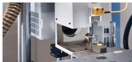
<p>The TruMark 5010 laser first removed the insulating varnish from the copper wire. The coil was then contacted.</p>
