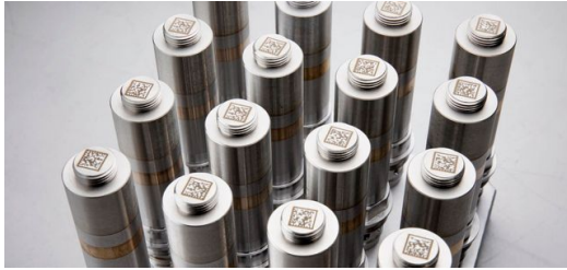
<p>The labeling of components with matrix codes is used for internal traceability of process steps.</p>
