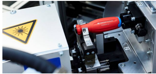
<p>Thanks to the integration of the marking system into an automated assembly line, a screwdriver is fully assembled and marked every five seconds. </p>
