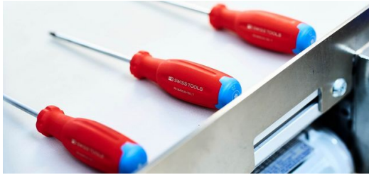
<p>To ensure you can quickly find the right tool, the laser marks the end caps of the tools with the symbol of the respective screw profile.</p>
