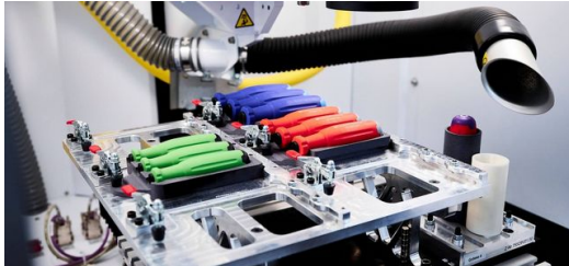
<p>Thanks to the marking laser, employees no longer have to label the handles by hand.</p>
