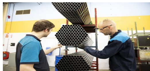
<p>Stainless steel tubes form the basis for the chairs by Ahrend and Gispén. They are usually round, rectangular, or oval. </p>
