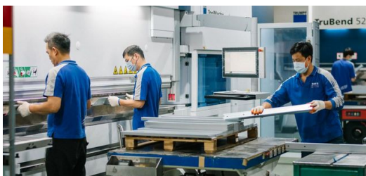
<p>Every single part of a C-bracket must be prepared with precision. INTER-TECH uses a wide range of bending machines from TRUMPF for bending.</p>
