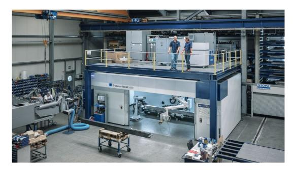
To save space, all the TruLaser Weld 5000's peripherals and system technology are positioned on a dedicated enclosure above the machine.
